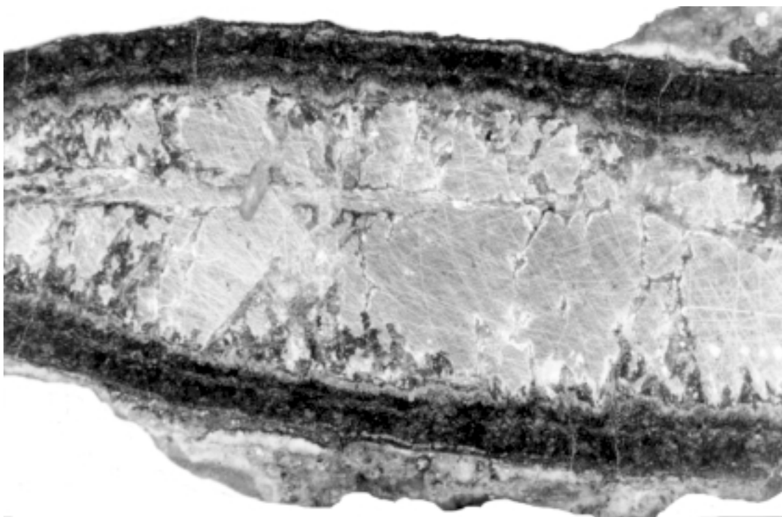
Figure 6. Microphotograph of a cross-section of the 210-2 oblong tin ingot corrosion pustule showing surface deposits of calcium carbonate and quartz. A layered crust is also seen (0.1 cm thick) which contains a darker layer of romarchite and a lighter layer of cassiterite. The core was composed mainly of relic metallic tin and interstitial abhurite. Approximate magnification x 11.
