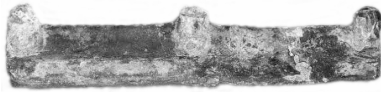
Figure 3. A macrophotograph of the pewter rod 210-3 showing the white deposits of cotunnite [ \text{PbCl}_2 ], laurionite [ \text{PbCl}(\text{OH}) ], cerussite [ \text{PbCO}_3 ] and traces of dark plattnerite [ \text{PbO}_2 ]
